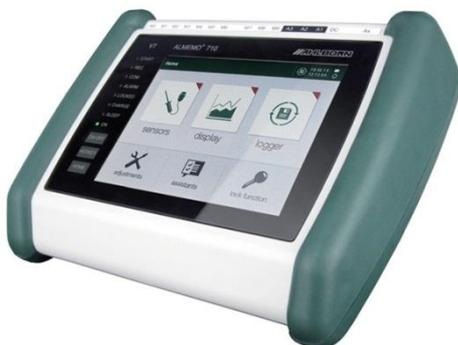
Fig. 7. Ahlborn Almemo 710 mobile measurement module [11]
