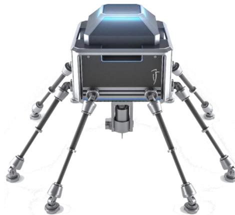
Fig. 1. Concept model of Picum One mobile milling machine [1]
