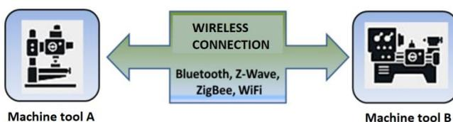
Fig. 3. Concept of cooperation (M2M) of technological machines
