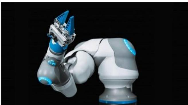
Fig. 10. Bionic-Cobot – a collaboration robot produced by Festo [14]
